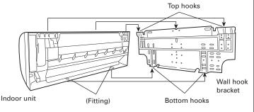
After hooking the indoor unit to the top hook, hook the fittings of the indoor unit to the two bottom hooks while lowering the unit and pushing it against the wall.
