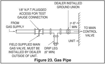
**Note:** The shut-off gas cock must be installed outside of the unit and should meet the specifications of all applicable national and local codes.
