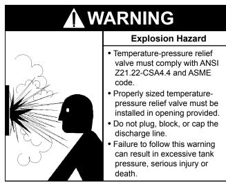
This water heater is provided with a properly rated/sized and certified combination Temperature-Pressure Relief Valve (T&P valve) by the manufacturer. The valve is certified by a nationally recognized testing laboratory that maintains periodic inspection of production of listed equipment of materials as meeting the requirements for **Relief Valves for Hot Water Supply Systems, ANSI Z21.22-CSA 4.4**, and the code requirements of ASME.
