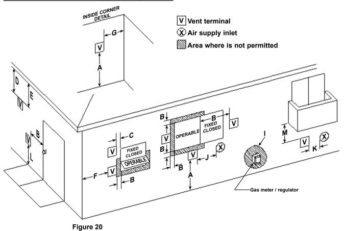
Vent terminal clearances for "Power Direct Vent" installations.
