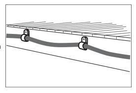
**Important:** When running Zurn PEX tubing, be sure to keep it away from potential sources of heat. Maintain a minimum of 12 inches between Zurn PEX and any recessed light fixture and a minimum of 6 inches between Zurn PEX and any gas appliance vent.
