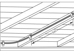
Always cut the pipe longer than necessary to allow some slack for any contraction in the pipe. 1/8" per foot of length is usually enough.
