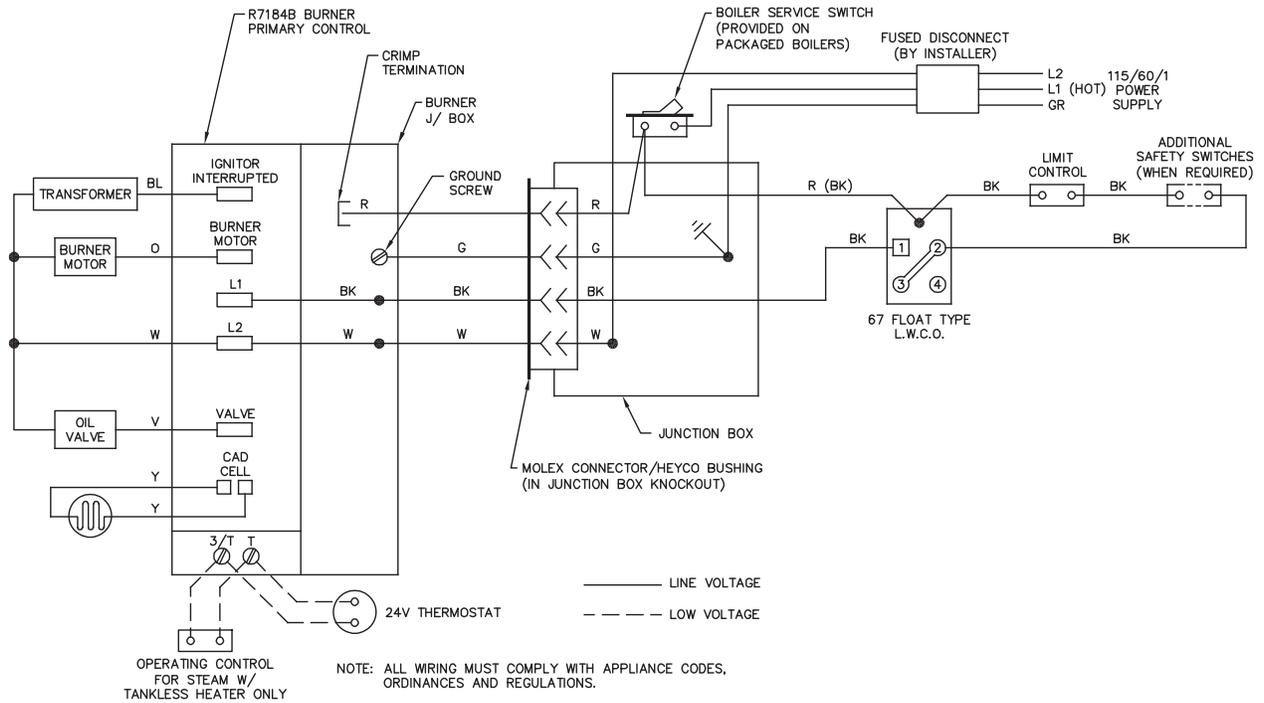
**Figure 4.6: Steam with Float Low Water Cut-off**
