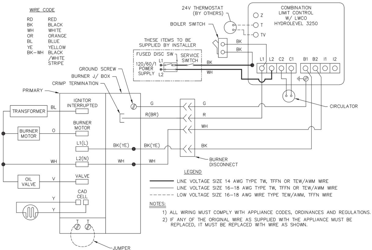
Figure 4.5: Water Boilers, Hydrolevel 3250 Limit Control
