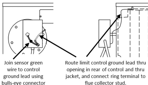
**Figure 4.1: Connecting Ground Wire on Beckett Limit Control**
