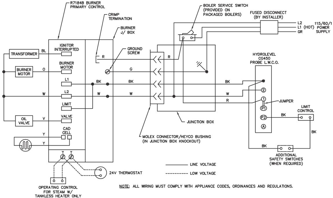
**Figure 4.7: Steam with Probe Low Water Cut-off**
