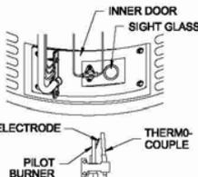
8. Turn the gas control knob counterclockwise
