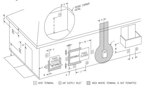
Figure 1 – Direct Vent Terminal Clearances
