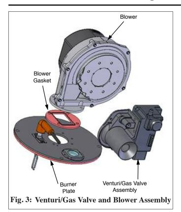
11. Attach the Molex plug(s) on the wiring harness to the connector(s) on the blower.
