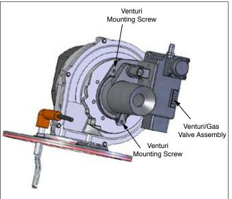
Fig. 2: Venturi/Gas Valve Assembly
