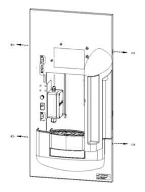
**Step 4:** Firmly screw filter cartridge into filter head (see Step 4 Diagram). NOTE: Bottle filler will work only if a filter cartridge is installed and its wiring is plugged in (see Step 9).
