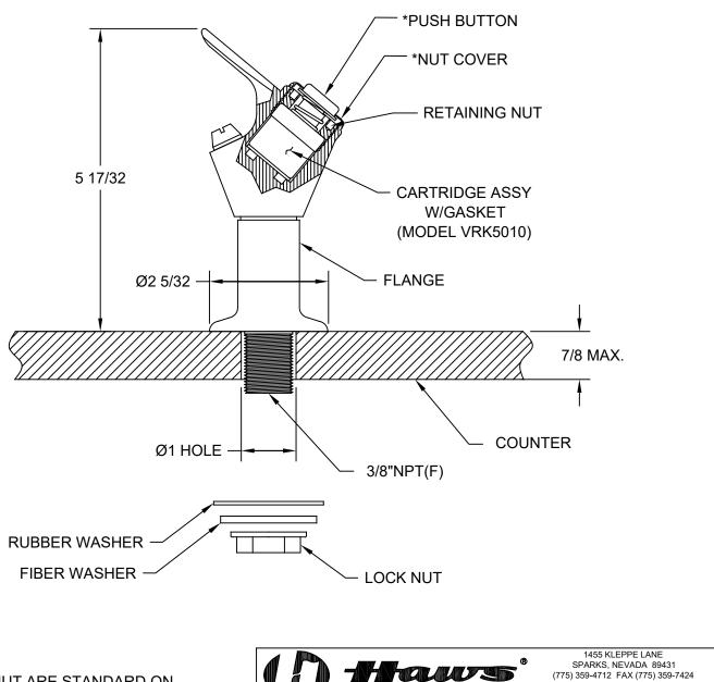
\*CHROME PLATED PUSH BUTTON COVER & NUT ARE STANDARD ON 5010.6427SS. COPPER PLATED OPTION IS AVAILABLE AS MODEL PB8C.
