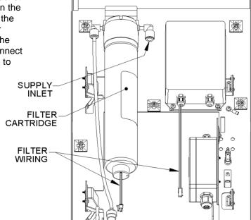
Step 8: Replace the mounting screws removed in Step 2 (see Step 2 Diagram for details). Provide AC power to unit.
