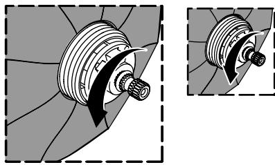
**23** Attach the stem adapter. Begin with the standard wall installation. Attach the handle. If the stem adapter is too long or the handle bonnet is not tight against the escutcheon, turn the stem adapter around and try the shallow wall installation.
