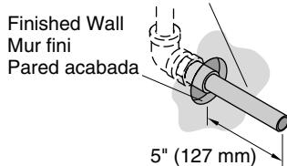
**Warning:** Tubes extending less than 4-5/8" (117 mm) will leak.
