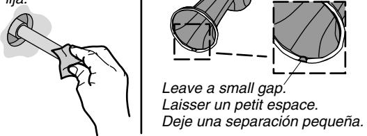
**3** Apply plumbers putty or sealant to the spout.
