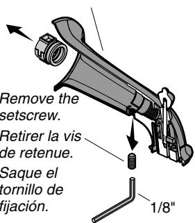
**4** Thread the spout onto the pipe.
