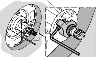
For minor temperature changes, adjust the setscrew and recheck the temperature.
