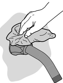
Remove the excess sealant.
