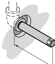
The nipple should extend 5" (127 mm) past the finished wall.
