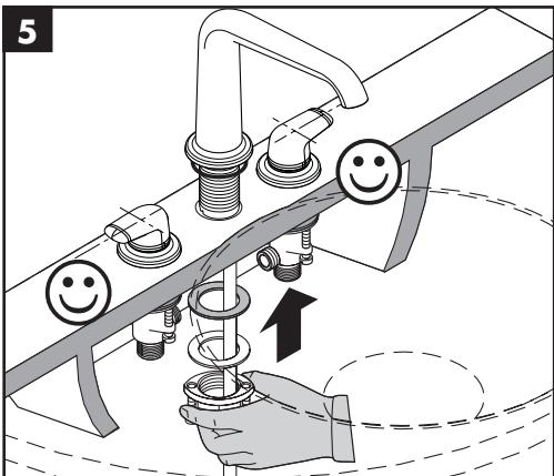
Position the spout and sealing ring on the mounting surface.
