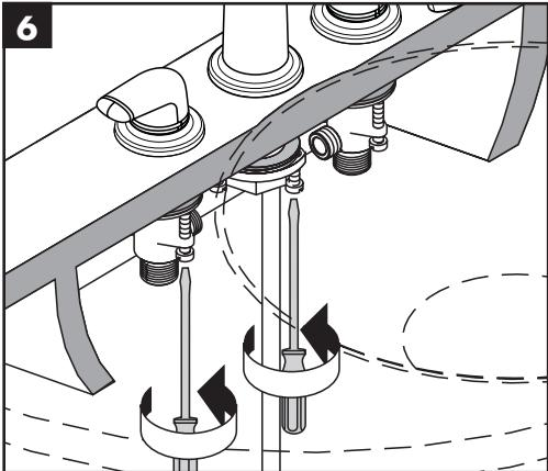
Tighten the tensioning screws.
