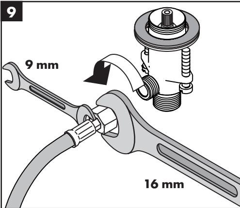
Connect the hot and cold connecting hoses to the valves.
