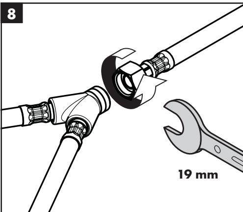
Connect the spout hose to the mounting angle.
