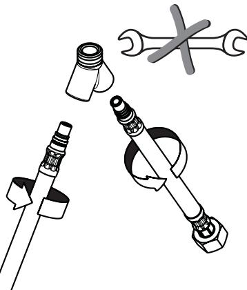
Install the hot and cold connecting hoses on the mounting angle.
