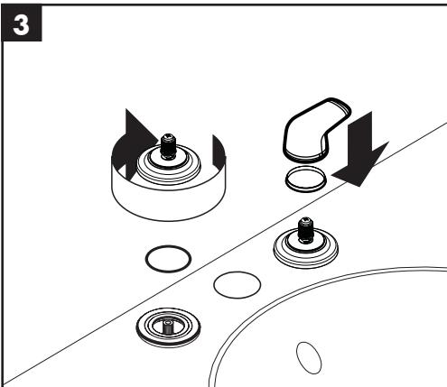
Rest the valve on the mounting surface.
