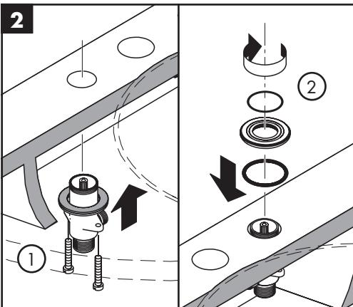
Install the metal washer and fiber washer on the valve.
