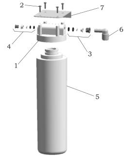
WATER FILTER EXPLODED VIEW <u>FIG. 7</u>
