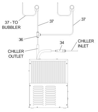
Figure 18 - OVL-II SER-Q/ESR-Q Tube Routing
