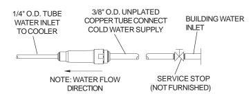
Figure 5 – Water Supply Connections
