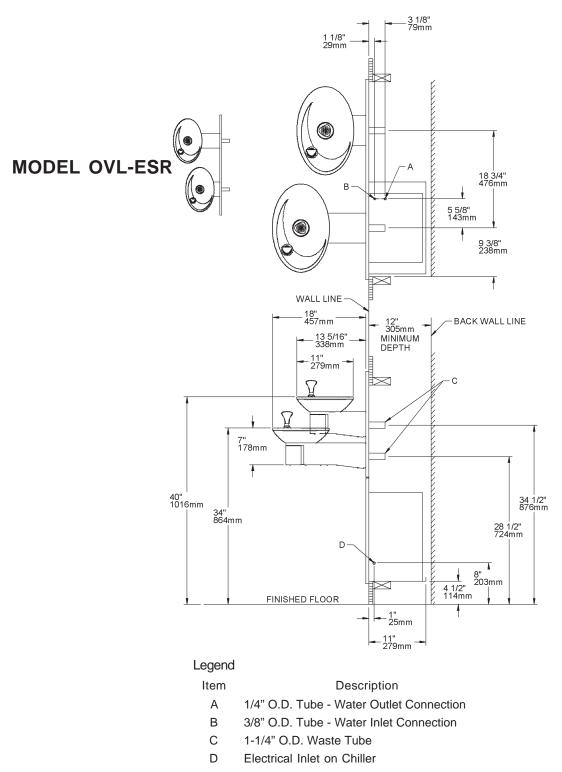
Figure 8 – OVL-II SER-Q/OVL-II ESR-Q Rough-In Dimensions
