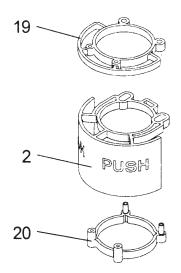
Figure 23 - Push Arm Mechanism
