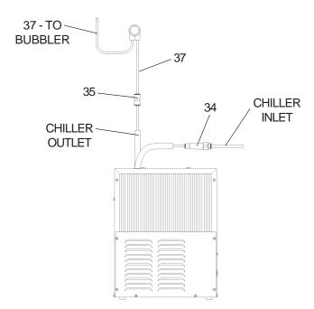
Figure 17 – OVL-II ER-Q/SR-Q Tube Routing
