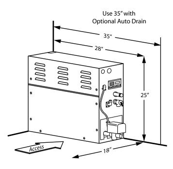
Select a location for mounting the Steam Generator that is accessible for installation and service. The access requirement indicates the minimum space for convenient access to Steam Generator.
