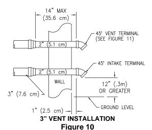
Vent terminal configurations for through the wall venting.
