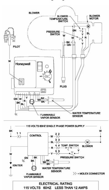
IF ANY OF THE ORIGINAL WIRES SUPPLIED WITH THE APPLIANCE MUST BE REPLACED, IT MUST BE REPLACED WITH APPLIANCE WIRE MATERIAL WITH A MINIMUM TEMPERATURE RATING OF 105°C AND A MINIMUM SIZE OF NO. 18 AWG.
