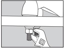
3. Tighten the nut on the hinge post using a wrench. **Caution**: Do not over-tighten the bolts as it could crack the toilet bowl.
