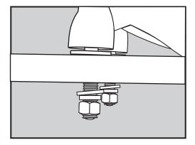
2. Properly align the toilet seat and install the metal washer, metal lock washer and metal nut onto the hinge post.
