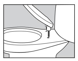
1. Insert the hinge posts into the bowl bolt holes making sure that the soft rubber washer is beneath the hinge and on top of the toilet bowl.
