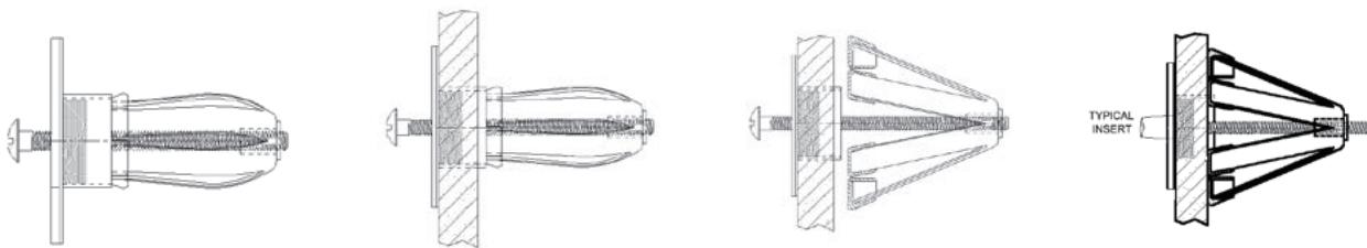
**2.1 Locate the 1-1/4 inch mounting holes so that the center of the grab bar fastener slides into the holes.**
