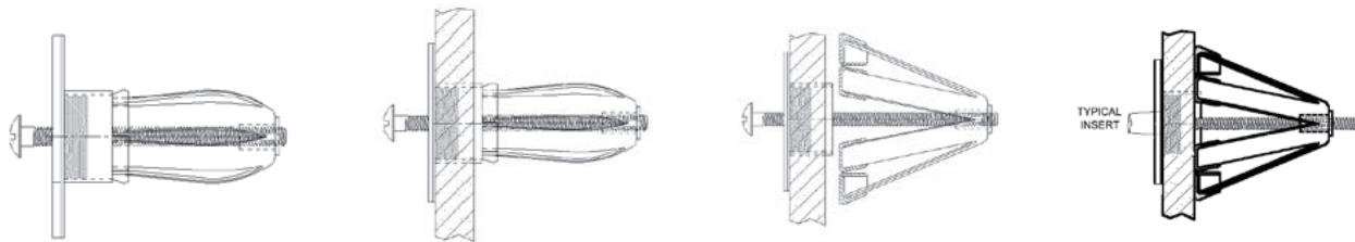
2.13 Remove the grab bar from the fasteners and use a screwdriver to firmly and quickly punch the head of the bolt toward the faceplate. You can also hit the screw gently but firmly with a rubber mallet or hammer.
