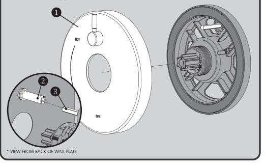
Align Handle Assembly with Connector (1) and Escutcheon as shown below. Keep Handle (2A) in a stationary vertical position and place over Connector (1) and engage the Splines of the Connector with the Handle Assembly. Keep Handle in the vertical position as you thread Handle Hub (2B) on to Mounting Base. Tighten until snug.
