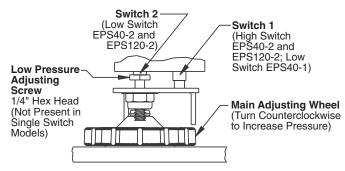
NOTE: Each 1/2 turn of Low Pressure adjusting screw adjusts pressure approximately 5 psi. Turn counter clockwise to increase pressure. Turn clockwise to decrease pressure. Each 1/2 turn of High Pressure adjusting wheel adjusts pressure 11 psi on the EPS40-2 and 40 psi on the EPS120-2.
