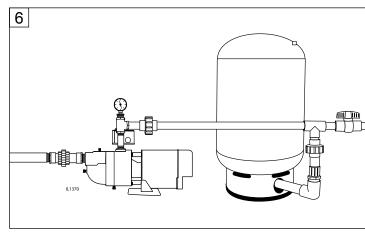
7. Optional tank mounted system is shown. Connections are basically the same as explained in previous steps. (**Fig. 7**)
