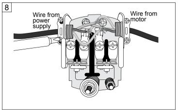
9. Connect the two wires from the power supply to the two outside terminals on the pressure switch. (**Fig. 9**)
