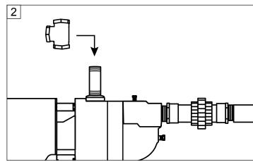
3. Install a 3/4 in. MPT x 1/4 in. FPT galvanized bushing and pressure gauge (optional), or a pipe plug. Do not tighten, as you will prime your pump later at this location. (**Fig. 3**)
