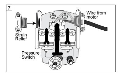
8. Thread the cable from the power supply through the strain relief and tighten both screws on the strain relief. Do not crush wire. (Fig. 8)
