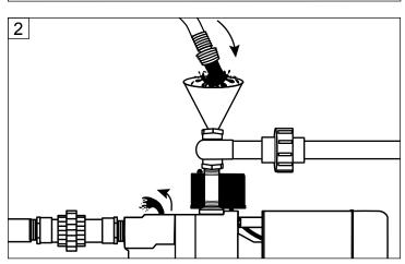
3. Replace air relief plug and continue adding water to pump cavity until water reaches the top of the priming plug. (Fig. 3)
