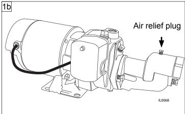
2. Slowly fill pump cavity until water comes out of air relief hole on top of the pump. (**Fig. 2**)
