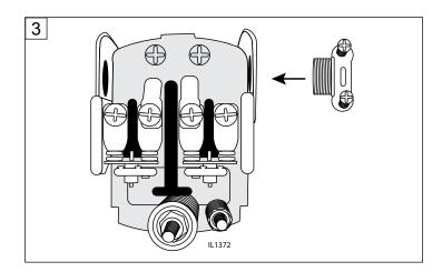
4. Thread the cable from the pump motor through the strain relief into the pressure switch cavity and tighten both screws on the strain relief. Do not crush wire. (**Fig. 4**)
