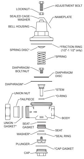
\* INDICATES PARTS SUPPLIED IN REPAIR KITS (spring disc not included in sizes 1 1/2" - 3")
