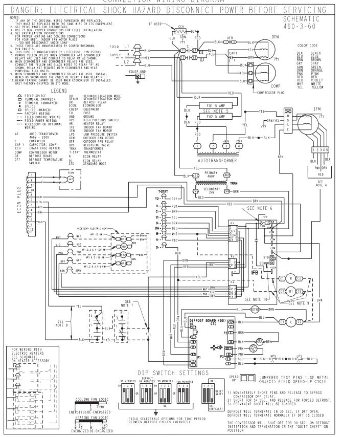
Fig. 16 - Connection Wiring Diagram 460-3-60
