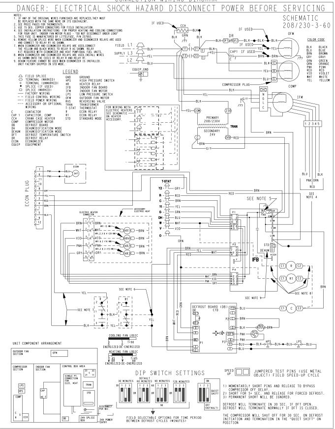
Fig. 15 - Connection Wiring Schematics - 208/230-3-60
