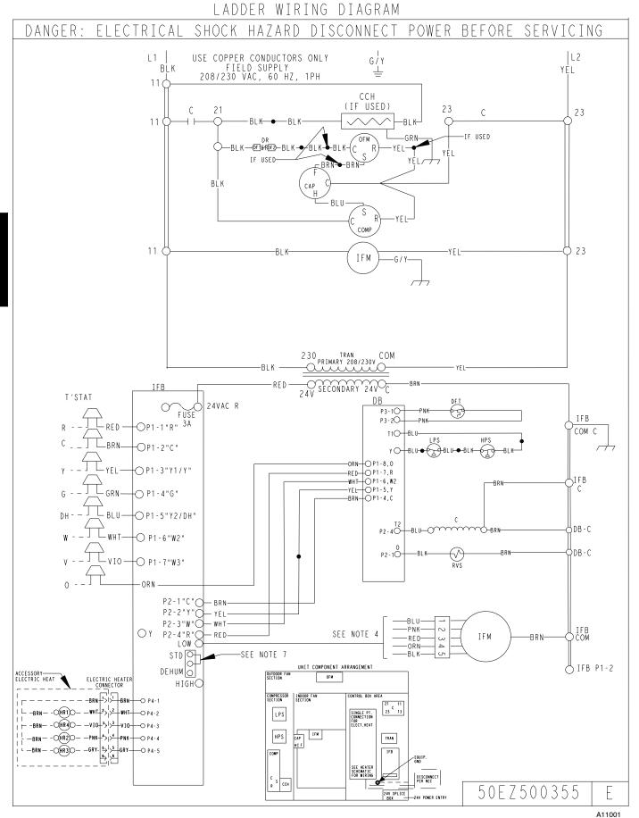
Fig. 12 Cont. - Ladder Wiring Schematics 208/230-1-60
