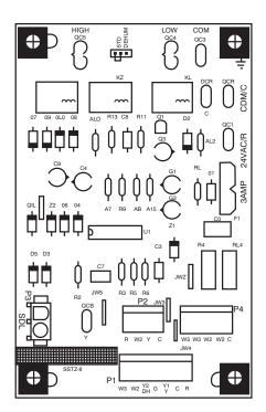
Fig. 18 - Interface Fan Board (IFB)
