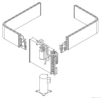
Fig. 22 - Refrigerant Circuit
