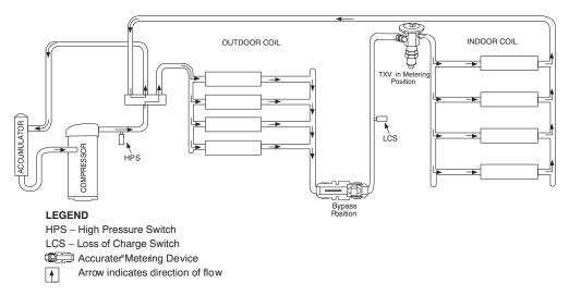
Fig. 17 - Typical Heat Pump Operation, Cooling Mode
