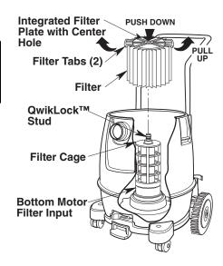
Align the small center hole in the top
