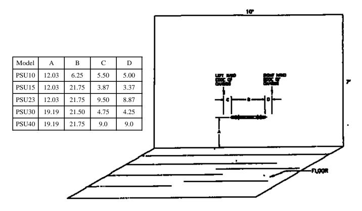
Make sure the fan convector is level and secure to the wall.
