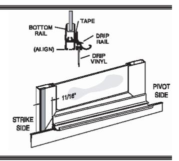
Adjust the drip vinyl [W] by sliding it left or right until it just touches the curb. Trim the vinyl (flush with the pivot end and notch <sup>1</sup>/<sub>4</sub>" longer than the drip rail as shown on the strike end). Secure it with one #6 x 3/8" truss head screw [E] in the pivot end of the drip rail.
