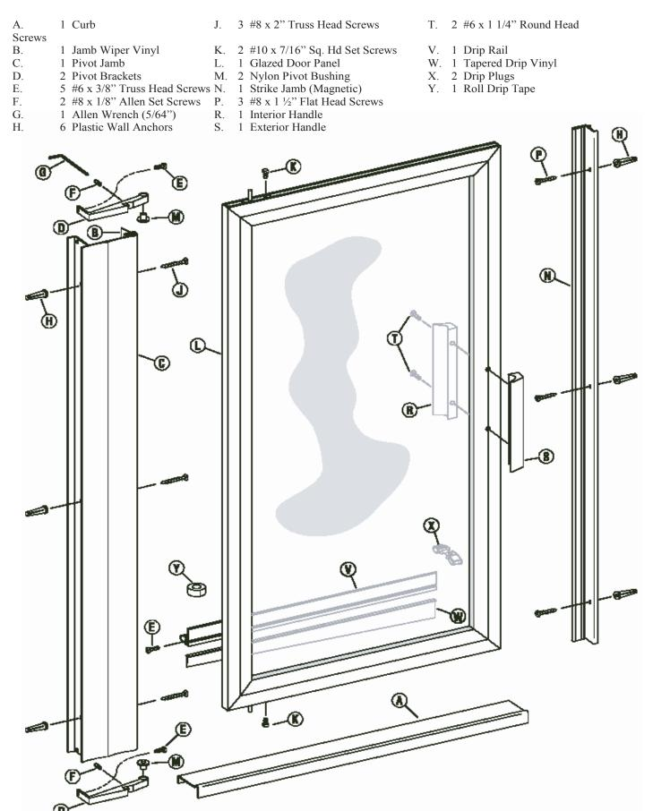
The Basco 100/200 Pivot Shower Door is completely reversible and may be installed pivot-right or pivot-left. Using the diagram, determine the correct position for your installation. For maximum waterproofing, the pivot jamb should always be opposite the shower head. These instructions depict a pivot left installation.
