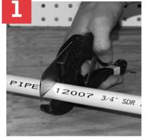
Acceptable tools include ratchet type pipe cutter,
