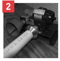
• Chamfer (bevel) the end of the pipe 10° - 15°.
