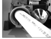
Sand outside corner of pipe around entire diameter using sanding sponge for a minimum of 20 seconds.
