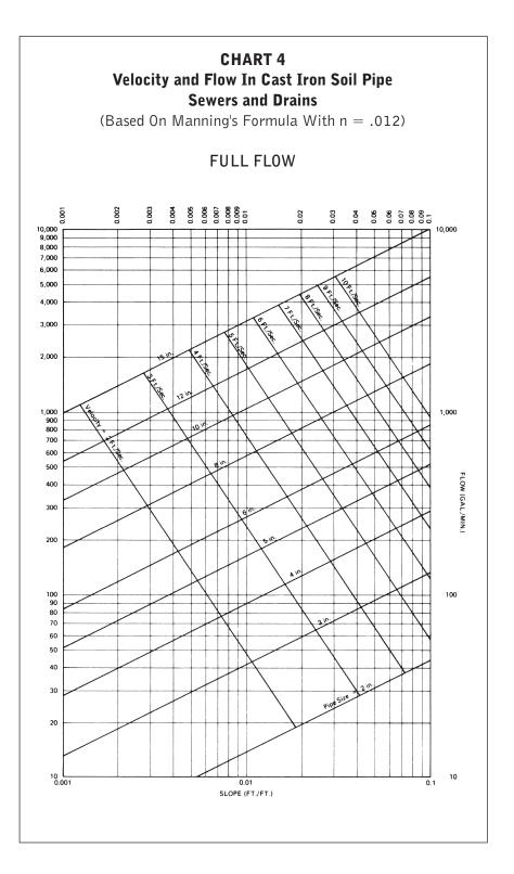
peak flow, which is usually based on population trends and area development over a period of fifty or so years. This requires that provision be made for any unforeseen increase in runoff, and therefore, cast iron soil pipe hydraulic systems are most frequently designed for halffull operation at probable future peak flow. Greater or less than half-full operation can be employed, depending on design requirements and the relative accuracy with which future flow can be forecast.
