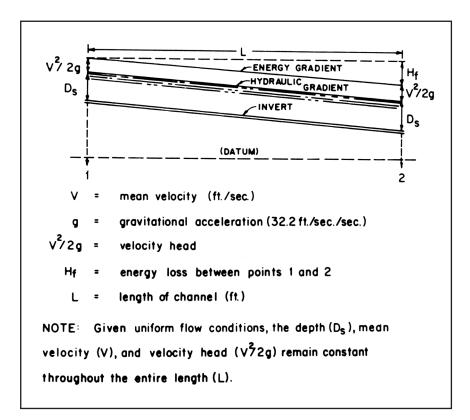
FIG. 2 - Uniform Flow of Open Channel Sewer or Drain
