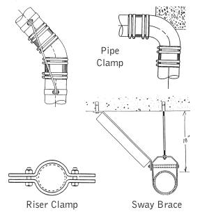
2. When installing large-diameter horizontal piping (five inches or larger), substantially brace the system to prevent horizontal movement. Use sway bracing as needed to stabilize side movement of the piping system. Use blocks, rods, bracing, or other suitable methods at each branch opening or change in direction. Different types of bracing are shown above.
