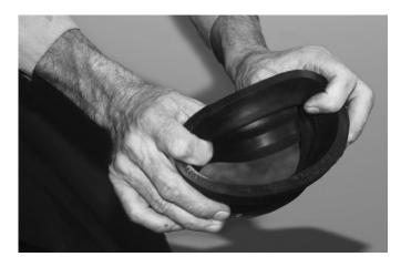
• **Thumb Fold:** Hold the outside circumference of the gasket and press thumbs down and in, as though turning the gasket inside out. Place the gasket into the hub and release it, allowing it to snap into proper position.
