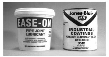
About Pipe Joint Lubricants: Regular lubricant is a flax-based compound that makes joining easy. It lowers the amount of force needed to join components by reducing friction. When you need to join large-diameter (5" through 15") components, we recommend that you use adhesive lubricant. Adhesive lubricant contains a neoprene-based adhesive which helps bond the components being joined.
