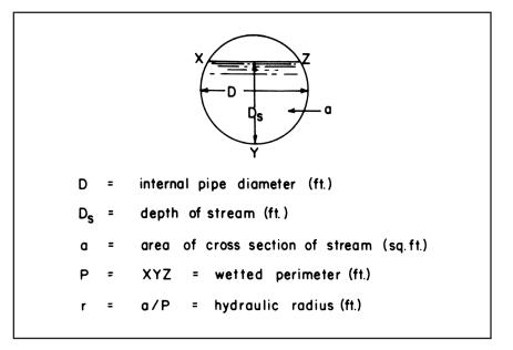
FIG. 1 - Cross Section of Cast Iron Soil Pipe Open Channel Sewer or Drain
