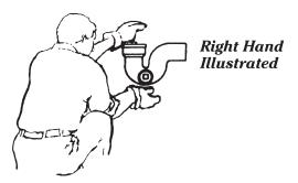
• **Closet Bends and P Traps** — Place the inlet upright near you, with the spigot facing away. If the side inlet is on your right, it is a right hand inlet.
