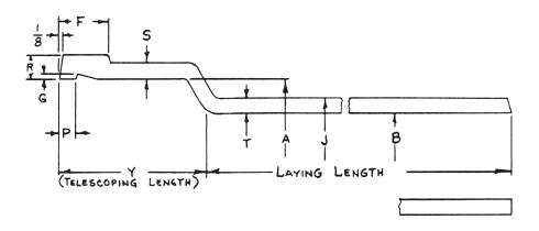
The tolerances set forth are intended for pipe and fittings designed for use with lead and oakum joints; however, these same tolerances may apply to pipe and fittings designed for use with a compression type gasket joint.
