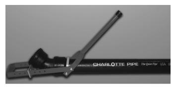
• Using Charlotte Pipe Part # EPT 920. Begin by installing the gasket into the hub as described earlier, lubricate, and then align the spigot. Next, place
