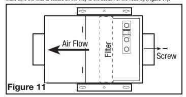
Close the access panel and reinstall the screw holding the access panel in place.
