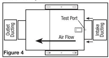
Ensure duct joints and exterior penetrations are sealed with caulk or other similar material to create an air-tight path to minimize building heat loss or gain and to reduce the potential for condensation. Place/wrap insulation around duct and/or fan in order to minimize possible condensation buildup within the duct, as well as building heat loss or gain.
