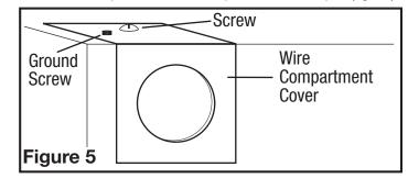
2. Pull the loose black, white and green wires out from the wire compartment (additional wires will be present). Install an approved electrical connector to the wire compartment cover (not included). Run a black (hot), white (neutral), and a green or bare ground wire from the supply through the electrical connector. Connect all wires from the supply to their corresponding wires within the wire compartment (Figure 6). Use approved methods for all connections.
