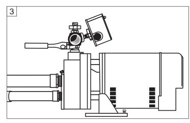
4. Install optional pressure gauge in 1/4" tapping on side of pump body. Face of gauge should be positioned so that dial can be read easily (Fig. 4).
