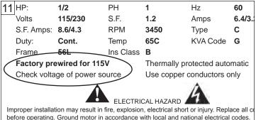
Improper installation may result in fire, explosion, electrical short or injury. Replace all of before operating. Ground motor in accordance with local and national electrical codes. Disconnect power source before touching internal parts. Motors equipped with automati protection may restart without warning.
