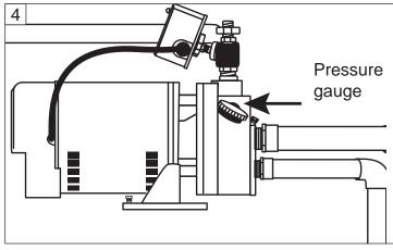
5. With pump operating at high pressure, open two or more faucets and slowly unscrew the flow control screw until maximum flow is obtained. This steady pressure will be minimum operating pressure and should agree with the pressure shown below. The flow control screw diverts the proper amount of water to operate the ejector. (Fig. 5)
