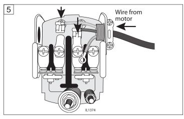
Connect the green ground wire from the motor cable to one of the green ground screws at the bottom of the pressure switch. (Fig. 6)
