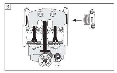
4. Thread the cable from the pump motor through the strain relief into the pressure switch cavity and tighten both screws on the strain relief. Do not crush wire. (**Fig. 4**)
