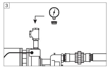
4. Continue with fittings and pipe to the pressure tank. A 3/4 in. union (optional) for easy connection and disconnection. (**Fig. 4**)
