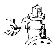
2. Replace packing injector screw.
