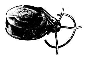
If the stop is frozen, pry the indicator stop out of the housing after unlocking it with the set screw or screws. If the valve must be turned before cleaning any rust or paint from the stop, use extreme caution to turn it in the correct direction to prevent disconnecting the gears or putting the connected grooves into the pipe. The keyway in the stem is parallel with the port opening in the plug. (See Sealant System on page 5.)
