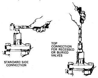
Step #1: Start coupler onto the fitting until the fitting head stops at the check valve (approx. half way).
