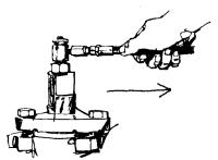
Step #3: Pull coupler onto the fitting with a gentle sliding movement. Reasonable care of sealant equipment will pay dividends in maintaining performance.
