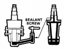
This superimposed drawing of a Nordstrom plug shows application of Pascal's Law. The Sealant screw, when turned, exerts powerful hydraulic force which will slightly raise the plug from its seat if necessary.
