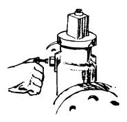
3. Tighten the packing injector screw to inject packing around the stem.
