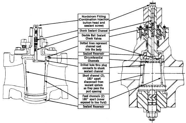
In the full open or closed position, four grooves are fed by the sealant reservoir. In other than the full open or closed position the two "feed" grooves are always connected to the reservoir.
