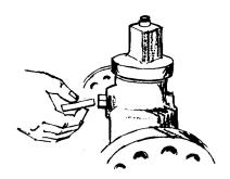
1. Remove packing injector screw. Insert a new piece of stem packing into the fitting.
