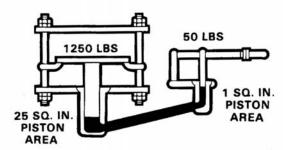
Here is a demonstration of Pascal's Law. A given pressure of 50 lb. lifts 1250 lb. over an enlarged area of 25 to 1 ratio.
