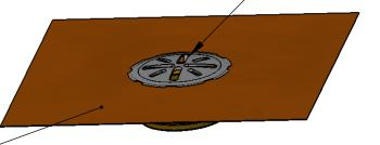
16 OZ. COPPER FLASHING ATTACHED TO 2", 3" OR 4" BRONZE FITTING. (2" THREADED FITTING ALSO AVAILABLE.)
