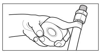
Figure 4-3A Wrapping with self bonding silicone tape - begin on jacket.
