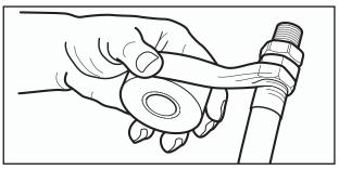
Figure 4-3B Wrapping with self bonding silicone tape - end on nut.
