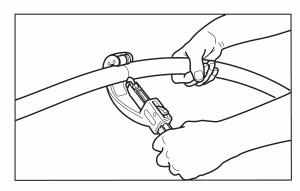
Unreel pipe into trench or on the ground and cut to desired length-plus one foot. Cutting up to 1" size can be done with a large tubing cutter. For 1-1/4" - 2" sizes, a reciprocating saw is recommended.
