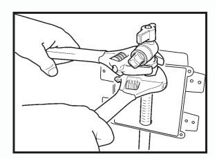
5. Thread 90 degree ball valve onto nut and tighten so valve outlet faces forward. It is recommended that crescent wrenches be used to avoid damaging valve or nut.
