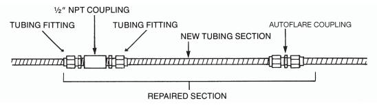
Figure 5-4 – Repair of Damaged Tubing with a New Section of Tubing and a joint splice or an AutoFlare Coupling
