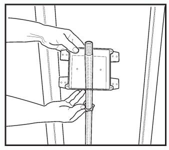
2. Remove box cover and slip locknut and box over end of pipe.
