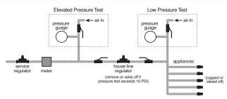
Figure 6-1 – Pressure Test Requirement for a 2 PSI System
