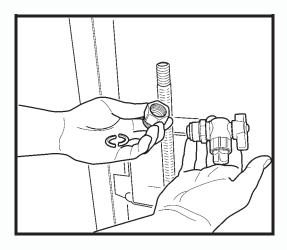
3. Disassemble valve and split rings from nut.
