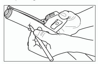
2. Mark the sleeve at specified length on the Strip Length Chart (below) - plus 2".
