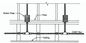
Figure 4-2 Multiple outlets along main tubing run
