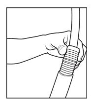
Insert a barbed coupling by sliding it over the exposed length of TracPipe and pushing firmly into the smooth black sleeve until all barbs are covered up to the coupling's center.
