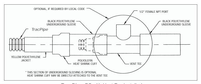
TracPipe PS with Vent Tee Installed Figure 4-20
