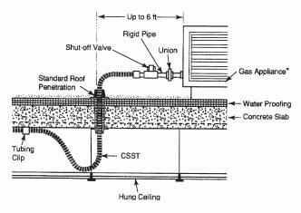
Figure 4-13 Short (1-6 foot) outdoor connection to roof mounted equipment
