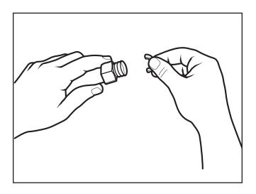
3. INSTALL FITTING NUT: Slide nut over cut end: place two split-rings into the first corrugation next to the tube cut. Slide nut forward to trap the rings.
