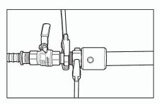
9. Thread nut onto adapter previously installed on the equipment. Using appropriate wrenches, hold adapter and tighten nut to proper torque specified. Do not over tighten or use any pipe dope or thread sealants on this connection. This is a metal-to-metal seat and will not seal if pipe dope or thread sealants are used. Sealants are to be used on the NPT connection to the equipment only!
