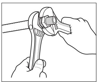
5. FINAL TORQUE: Tighten nut and adapter to the torque values shown in Table 4-3. For field installations use the following method: Tighten nut and adaptor as though you were making up a flared tubing joint. Note relation between hex flats at this point and continue to tighten for two additional hex flats (one-third turn) to obtain required torque and final leak-tight seal.
