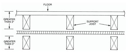
Figure 4-6 No Shielding Requirement at Support Area when Points of Penetration are greater than 3 inches from any Edge of a Stud, Joist, Plate, etc.
