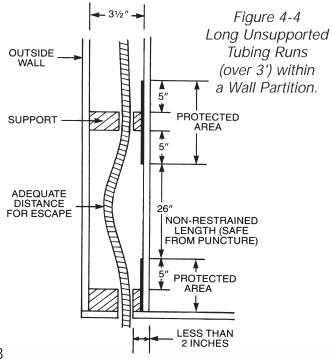
b. At support points and points of penetration 2 to 3 inches from any edge of stud, joist plate, etc. shielding is required throughout area of support. Use a quarter striker plate in these locations. (Figure 4-5) include: (but are not limited to) outside walls of buildings with sheathing in place, between floors with enclosed joist areas, and retrofits in existing buildings with walls in place. Steel pipe having an inner diameter at least one-
