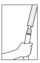
5. Slide cut section of flexible poly tube over the remaining barbs on the coupling.
