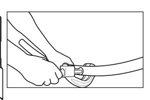
Cut through the smooth black sleeve using a Ridgid™ 151 or similar tube cutter of the appropriate size for the tubing. USE CARE: Do not cut through the yellow jacket or damage the stainless steel tubing inside.
