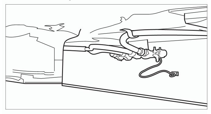
5. If a manifold is used, it shall be rigidly mounted to the I-beam flange. This applies to parallel system layouts. Gas pressure in HUD Code homes is limited to 14 inches water column maximum. Line pressure regulators are not necessary for this pressure and should not be used.
