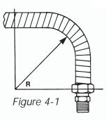
ed bend radius for general routing of tubing is listed in Table 4-1. Multiple tight bends can restrict the gas flow and increase pressure drop. The tightest bend allowed for each size of *TracPipe* is shown in the chart below. Typical locations
