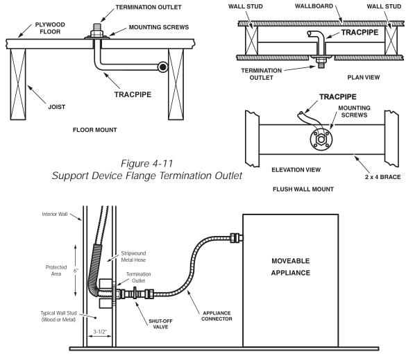
Figure 4-12 Stainless Steel Gas Connector Connection to a Movable Gas Appliance
