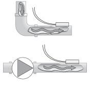
The stiff wire of the Universal Sensor 078 allows it to be inserted into deep temperature wells such as those found on domestic hot water (DHW) tanks.
