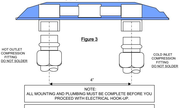
TEST THE INSTALLATION FOR LEAKS BEFORE CONNECTING THE ELECTRICAL SUPPLY.
