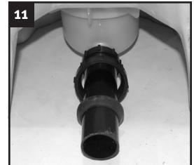
Install the extension tube onto the housing tail pipe and slide the 2" slip joint nut and washer onto the extension
