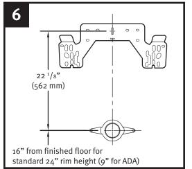
Measure and mark the rough-in. Use a 5/16" masonry bit to drill hole, then install he hanger bracket with one screw.
