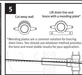
Adjust the drain to achieve pitch. Code requires a 1/4" drop per foot of drain line for proper pitch.
