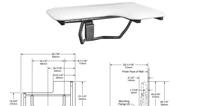
Base Plate Universal/Barrier-Free 7-1/4" 9-3/8" Recommended Mounting Height \*17" to 19" with Spring at Top 2-1/4" Guide Bracke 430 to 485mm Finish Face of Floor
