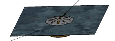
16 OZ. COPPER FLASHING ATTACHED TO 2", 3" OR 4" BRONZE FITTING. (2" THREADED FITTING ALSO AVAILABLE.)
