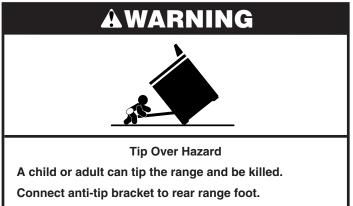
Reconnect the anti-tip bracket, if the range is moved.
