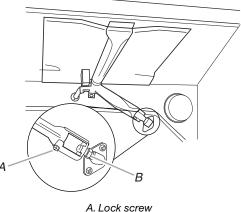
A. Lock screw B. Orifice hood
