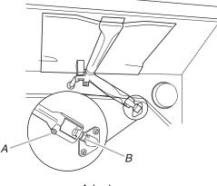
A. Lock screw B. Orifice hood
