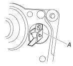
A. Gas pressure regulator shutoff valve
