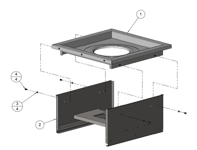
**NOTE:** AGVPC UNITS BUILT AFTER 07/2009 HAVE BODIES BUILT WITH TWO ASSEMBLIES, TOP (510-0448), ITEM 1 AND BOTTOM (510-0449), ITEM 2, MAKING THE TOP OR BOTTOM ASSEMBLIES REPLACEABLE BY THEMSELVES.
