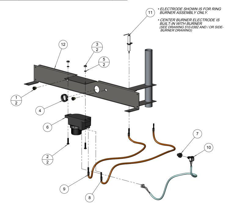
**NOTE:** ITEM 12 (ASSEMBLY 510-0398) IS SHOWN FOR ILLUSTRATION AND GENERAL ASSEMBLY PURPOSES ONLY. THIS ASSEMBLY IS ACTUALLY PART OF THE MAIN BODY ASSEMBLY 510-0378 SHOWN ON DRAWING 500-0063B
