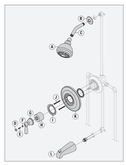
\*Note: Apply a bead of silicone around the perimeter of the escutcheon after installing trim flush with wall. Leave opening on bottom of escutcheon for weep hole.
