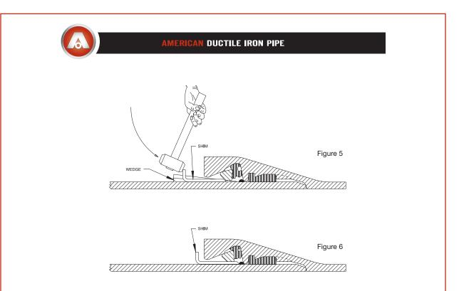
4. With a large hammer (such as a six pounder) vigorously drive one or two "L"-shaped shims under the locking segment until the ends of the shims firmly contact the spigot weld bead. (Fig. 5) Shims and wedges can be safely and firmly held against the pipe as they are hammered using a block of wood or a board. Safety precautions such as the wearing of safety glasses and keeping clear of the hammer during striking should always be taken to avoid injury.
