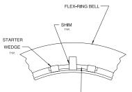
FLEX-RING SEGMENT — Figure 1 Starter shim and wedge arrangement for 14", 18", and 20" sizes.
