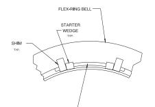
FLEX-RING SEGMENT — Figure 2 Shim and wedge arrangement for 16", 24", 30", 42", 48", and 54" sizes.
