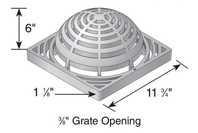
Material: UV Protected High Density Polyethylene (HDPE)
