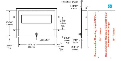
Rough Wall Opening 15-5/8" (395mm) wide 11-1/4" (285mm) high 2-5/8" (67mm) minimum recessed depth
