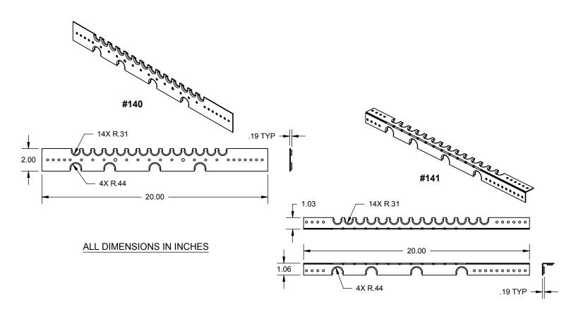
The HOLDRITE® #140 and #141 are Copper-Bonded™ steel brackets with 5/8" extruded notches on 1" centers and 7/8" extruded notches on 4" centers. #141 bracket is bent at 90° degrees in the middle for added strength. Solder copper tubing to the bracket.
