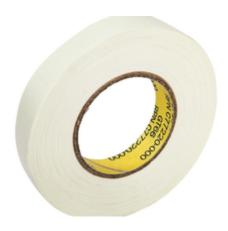
nVent RAYCHEM GT-66 is a glass installation tape to attach trace heating cables to pipes. For stainless steel, or when installation temperatures drop below 40 °F /5 C°, use GS-54 fixing tape. ATE-180 aluminum tape is used to attach heating cables and thermostat sensors to pipes and tanks.
