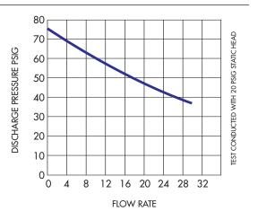
Note: Minimum Inlet Flow Pressure is 10 psig. Tank Pre-charge pressure is factory pre-set at 38 psig, Tank Maximum Working Pressure is 100 psig. Voltage is 115/230. Factory settings are for a water main pressure of 20 psig. To operate with lower water main pressure (minimum of 10 psig required), pressure switch and tank pre-charge must be adjusted. Note: The pressuriser is designed for cold water use.
