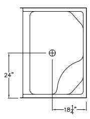
G 4800 SH TILE 1S. SHOWER UNIT HAS ONE LARGE MOLD SEAT, LEFT OR RIGHT, TWO MOLDED SOAP LEDGES, AND SIMULATED TILE SURFACE.
