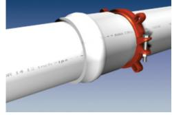
3. Install both halves of the serrated ring around the pipe behind the bell, tapping each half into place. Make sure that the complete ID of the ring is touching the pipe before installing the side bolts. Install the side bolts and tighten evenly to 110 ft-lbs. of torque. (60 ft-lbs on 4 inch and 6 inch)
