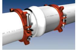
5. Install both halves of the restraint ring at the proper location, tapping each half into place. Make sure that the complete ID of the ring is touching the pipe before installing the side bolts. Tighten the side bolts evenly to 110 ft-lbs. (60 ft-lbs on 4" and 6")
