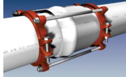
Place nuts on the thrust bolts and tighten until they are snug. Allow enough room on the thrust bolts to fully engage the nuts. Do not tighten these bolts enough to force the spigot further into the bell of the joint.
