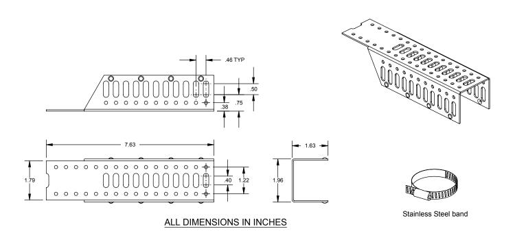
The HOLDRITE® #115 and #115-C (Copper-Bonded™) are steel brackets designed to position water supply lines off the vent or waste pipe in chase walls. Supports 1/2" through 2" pipes both vertically and horizontally. Packaged with self-locking stainless steel band, screws, metal clamps, and self-adhesive isolating felt. Excellent for pre-fab applications. Supports piping prior to wall framing. Heat the pipe, not the bracket when soldering the #115-C version.
